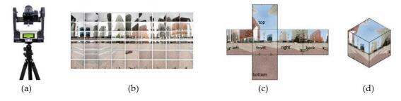
**Figure 7.** Procedure for creating immersive virtual environments: (**a**) Capturing, (**b**) stitching, (**c**) cube mapping, and (**d**) image wrapping.
